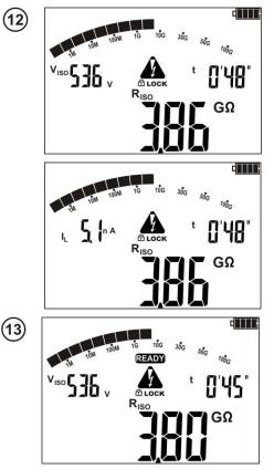
View of the screen during measurement. **IDCCK** means that the measurement was started with **ENTER** button or by pressing and holding **START** button for approx. 5 sec.
