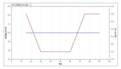
For a measurement with voltage increase method (RampTest), the user basing on performed measurements, may analyse the characteristics of voltage, resistance and current as a function of time.
