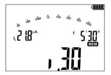
The value of leakage current  $I_L$  measured in time t=5'30'. Symbol  $J_{11}^{(1)}$  indicates the selected time interval, in which the leakage current value was recorded.
