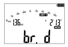
If the electric resistance strength of the tested insulation is ecceded and the puncture occurs, the main field of the display will show message br. d - breakdown.
